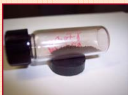
A dehydrated powdered alginate-nanoparticle sample as presented to our group. The ferro-magnetism of the sample is evident due to the small magnet the sample sits upon.
